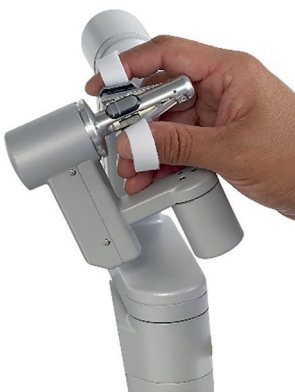
Fig. 8 The control unit which the surgeon would use to control the instrument
